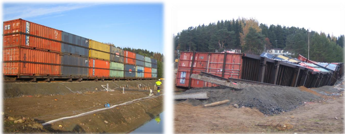
Figure 48. Containers simulating train loading at Perniö before (left) and after (right) failure.
