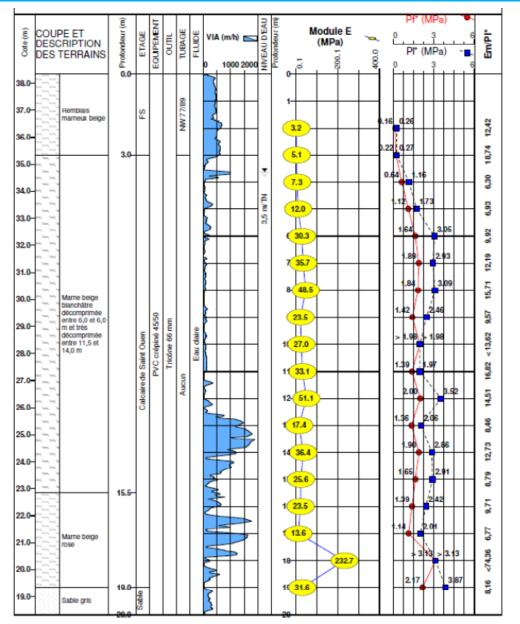
Results of pressuremeter tests between abutment C0 and pier P1
