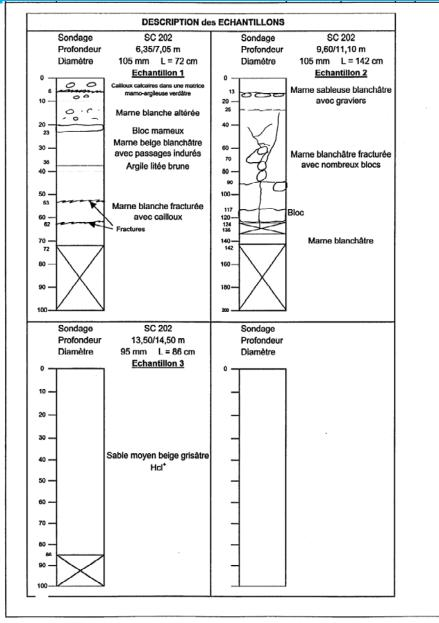
Identification of soils : core sampling results between abutment C0 and pier P1
