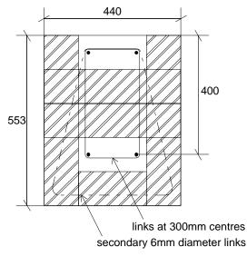
Figure: Steel arrangement in reinforced masonry beam Note to figure: substitute d as 410mm and not 400mm
