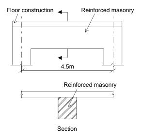
Figure: Elevation and section of reinforced masonry beam Note to figure: substitute a clear span of 3,80m instead of 4,50m structural span
