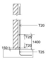
Figure: Steel arrangement in retaining wall Note to figure: for 1400 dimension substitute 2074
