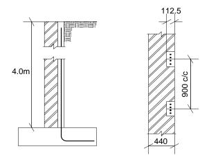
Figure: Design of brickwork wall stem Note to figure: substitute height of stem as 3,65m; wall trial thickness as 328mm
