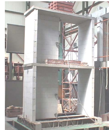
Test on shaking table in Athens (CS)
