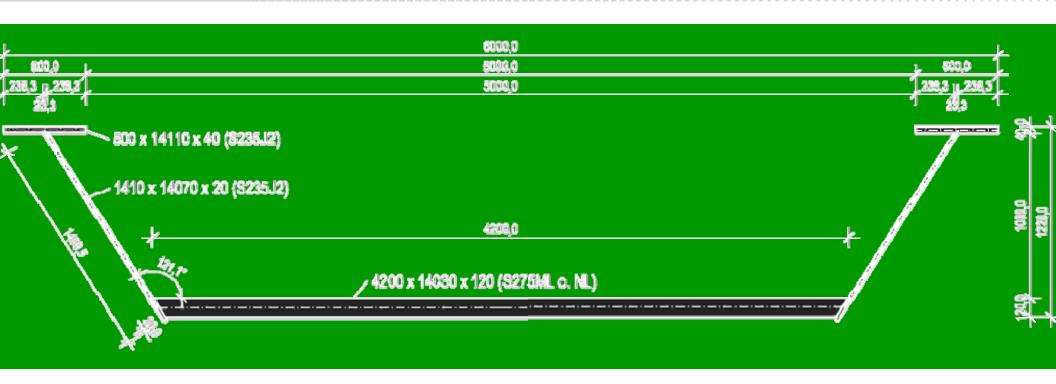
principle cross section for a span range of 10 - 20 m
