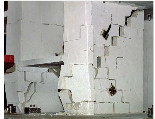
Damage grade 4: at 0.8 R_{max} (Model M2-2, R100/3, \Phi_u = 1,77 \% )
