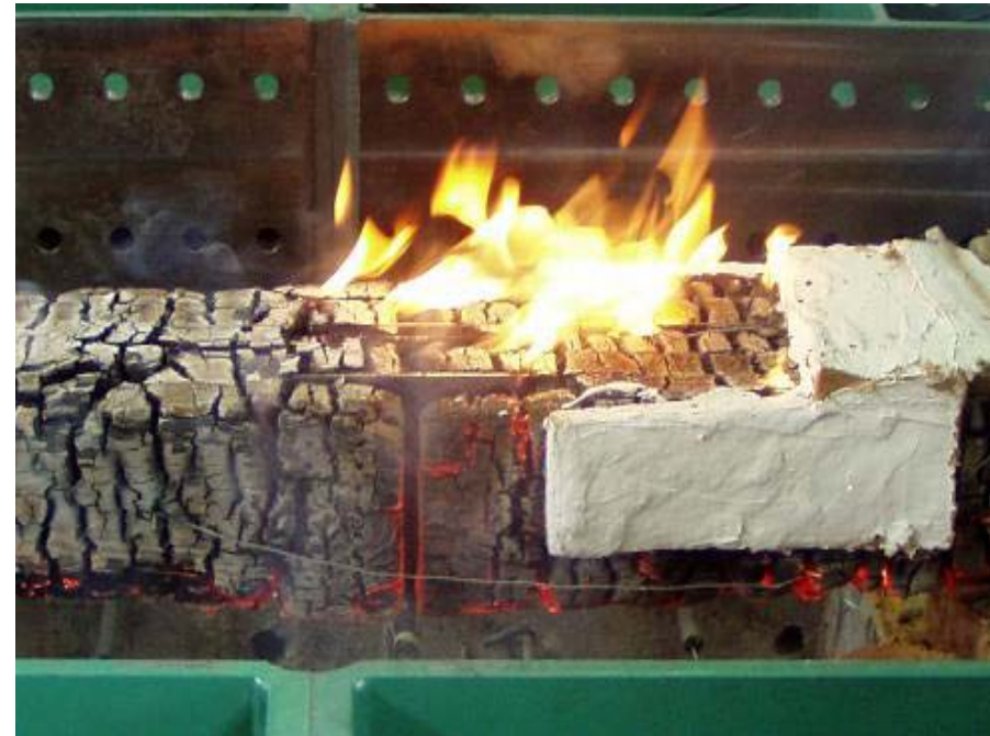
Multiple shear steel-to-timber dowelled connection
