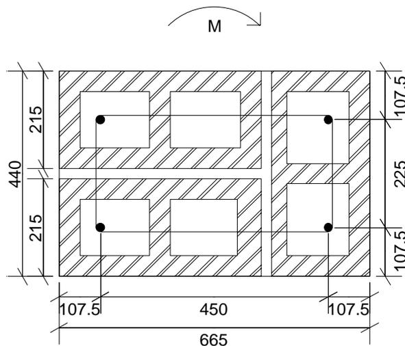
Figure: Steel positions in hollow concrete blocks
