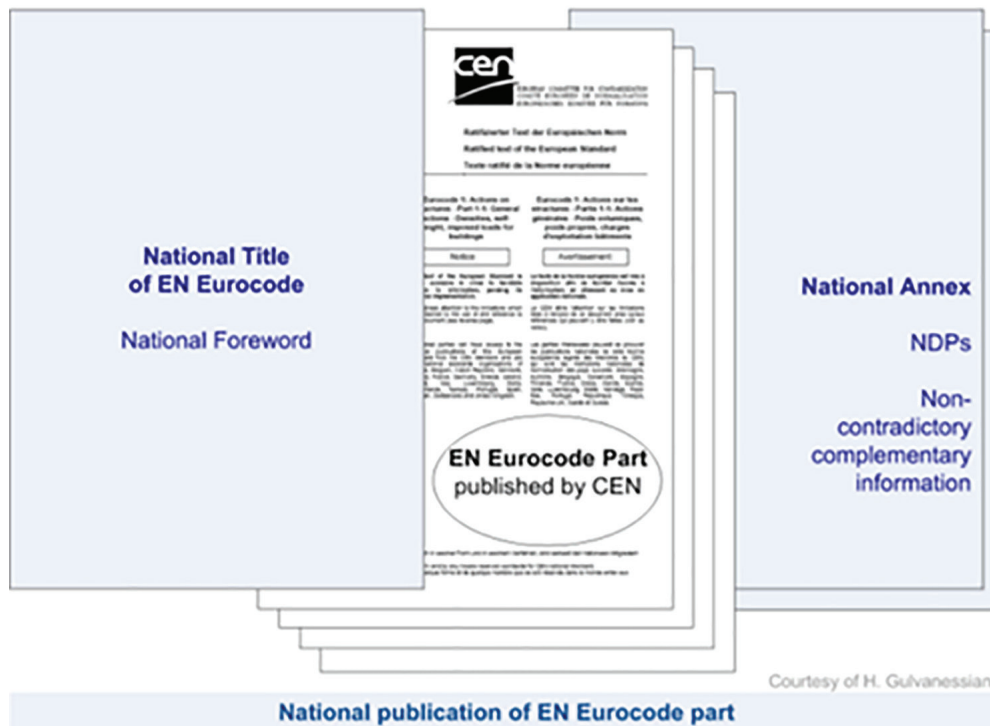
Figure 10. National publication of EN Eurocode part (source: National Standards | Eurocodes: Building the future (europa.eu) https://eurocodes.jrc.ec.europa.eu/en-eurocodes-implementation/national-standards?id=35 )
