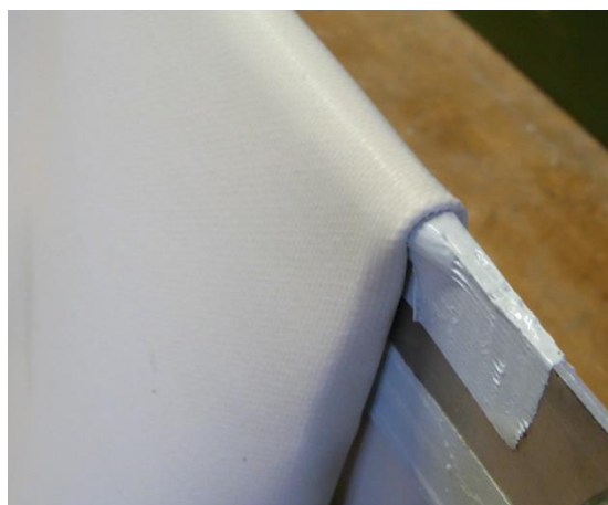
Figure B2-6 Procedure to create a running crease, lower part will be extracted by using a straight edge with a defined diameter [© DEKRA/Labor Blum]
