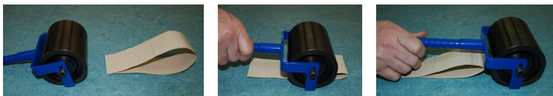
Figure B2-1 Preparation of the looped specimen for the crease fold test acc. to ASTM D4851-07 [© ELLF]
