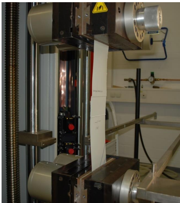
Figure B1-1 Tensile test specimen with welding seam in the testing machine before testing [© ELLF]
