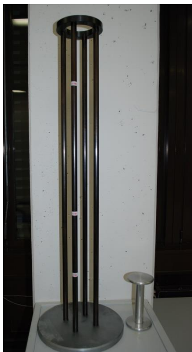
Figure B2-3 Left: loading device for the Essen method for repeated folding and force applications, right: rolling the load device on the looped end [© ELLF]
