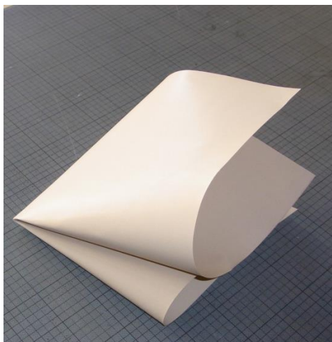
Figure B2-5 Procedure to create a running crease, specimen folded twice [© DEKRA/Labor Blum]
