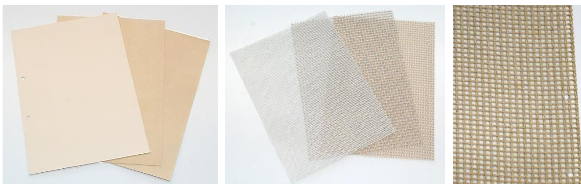
Figure 2-3 Main fabrics used in textile architecture [© ELLF]
