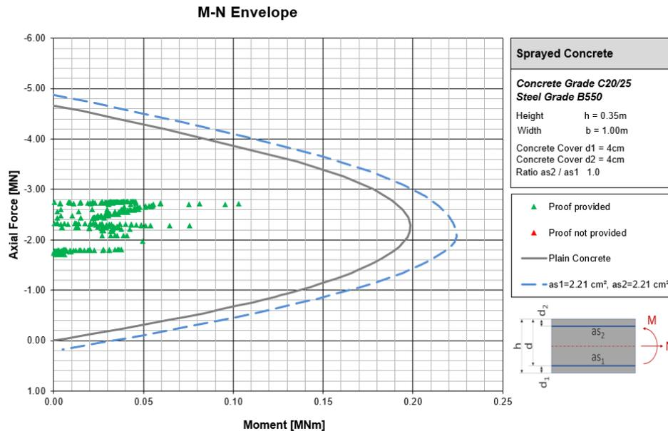
**Figure B1.10** M-N Envelope for the wire mesh reinforced concrete lining in the primary lining
