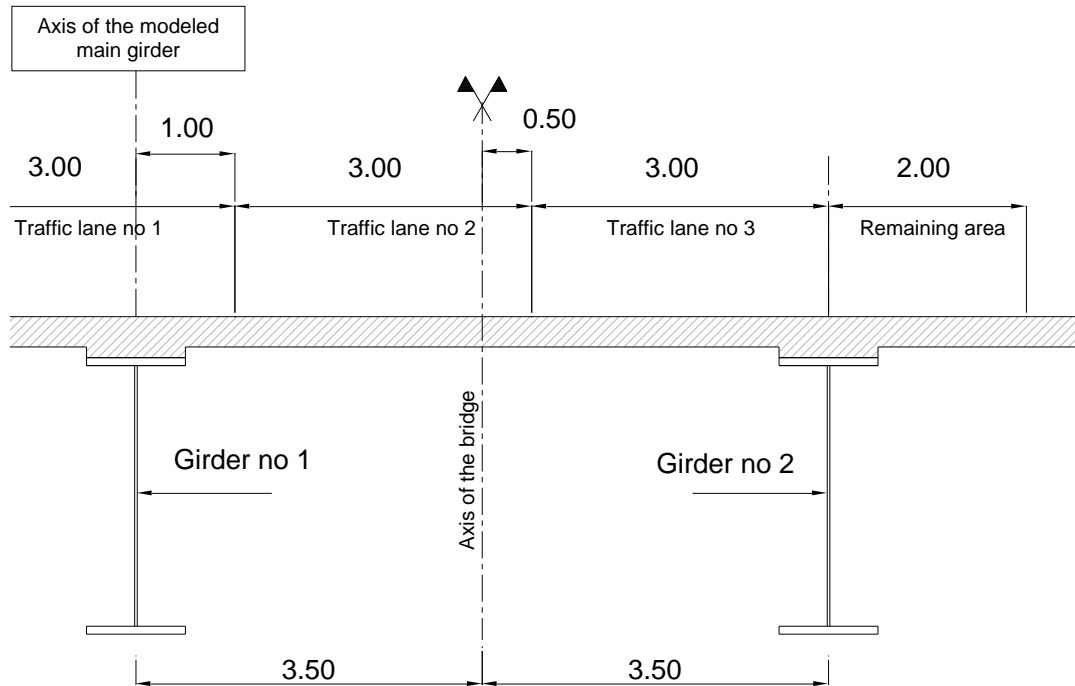
Figure 4.4 Transverse positioning of the traffic lanes
