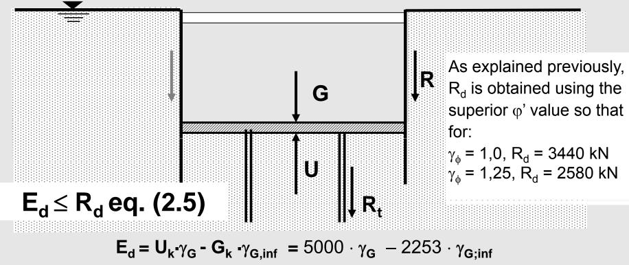
$$\begin{aligned} \mathbf{R_{t,d}} &= \mathbf{R_{t,k}} / \gamma_{s;t} + \mathbf{R_d} = \mathbf{L_{tot}} \cdot \mathbf{q_{s,k}} \cdot \pi \cdot \mathbf{D} / \gamma_{s;t} + \mathbf{R_d} \\ &= \mathbf{L_{tot}} \cdot 35 \cdot \pi \cdot 0.5 / \gamma_{s;t} + \mathbf{R_d} = \mathbf{L_{tot}} \cdot 54.98 / \gamma_{s;t} + \mathbf{R_d} \\ \text{Hence require: } \mathbf{L_{tot}} \geq \gamma_{s;t} (5000 \cdot \gamma_{G} - 2253 \cdot \gamma_{G;inf} - \mathbf{R_d}) / 54.98 \end{aligned}$$
