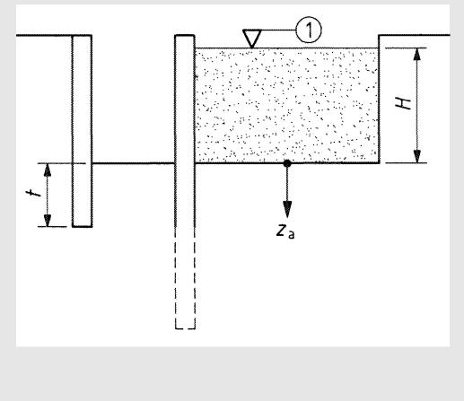
b) Where the piezometric surface and the **groundwater tables** are **above the excavation base**, the larger value of the following conditions should be met:
