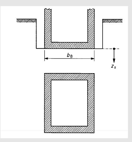
(6) For raft foundations and structures with several foundation elements whose effects in deeper strata are superimposed on each other:
