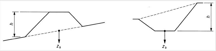
(7) **Embankments** and **cuttings**, the larger value of the following conditions should be met:
