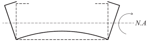
Figure 4.13 Flange curling of channel section beam
