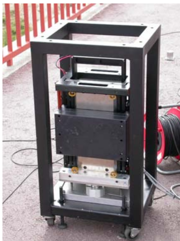
Figure 5-2: Electromagnetic shaker for civil engineering applications. Vertical mounting
