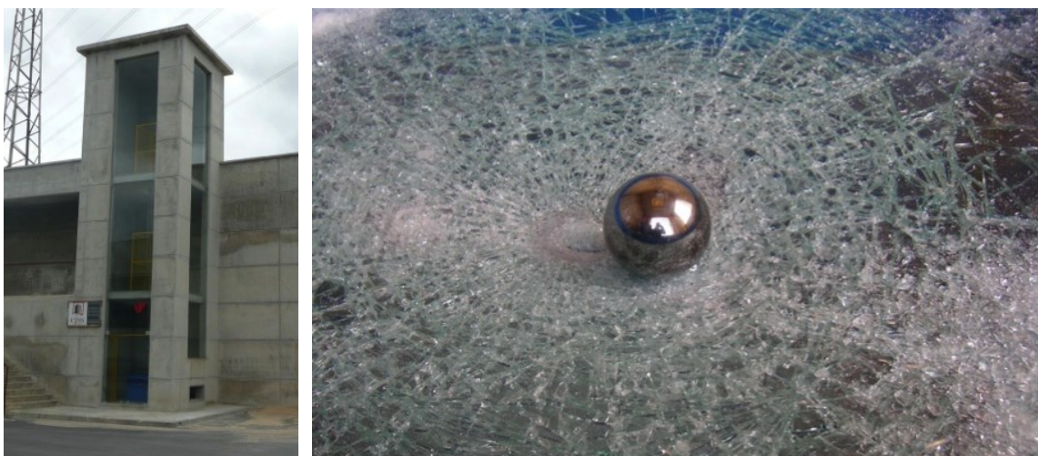
Figure 3-3 Test tower for 9 m high hard body drop and glass specimen broken but not perforated after hard body drop test [127]
