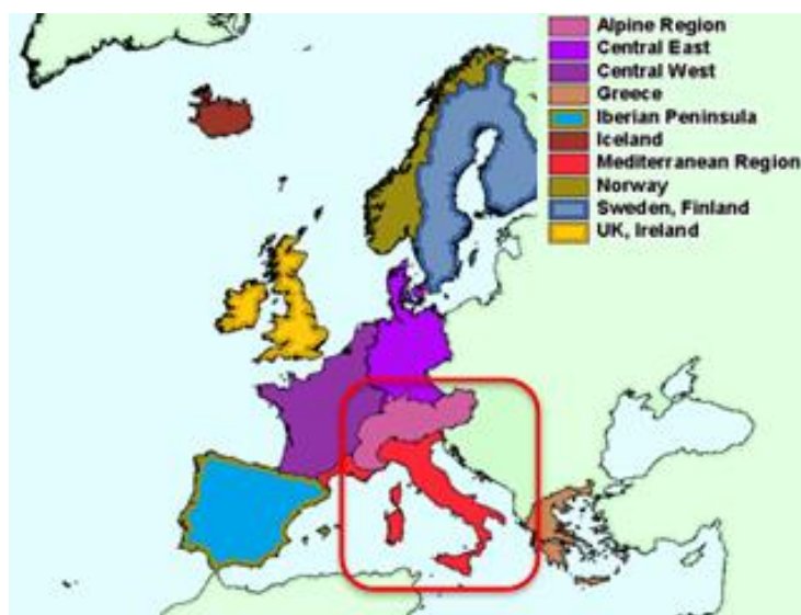
Figure 5.1 Major climatic Regions for snow loads; (adapted from Sanpaolesi et al., 1998 and 1999) [© CEN]
