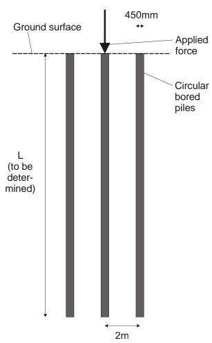
Figure 2.6a: Pile arrangement
