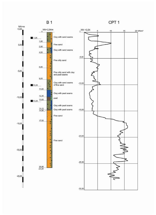
Figure 2.6b: Cone penetration resistance from CPT test
